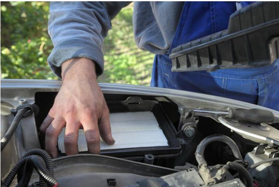
Replacing your old spark plugs and air filter can instantly improve engine performance and efficiency. Spark plugs should be replaced every 50,000 miles, whereas filters should be replaced as often as every 15,000-30,000 miles.
